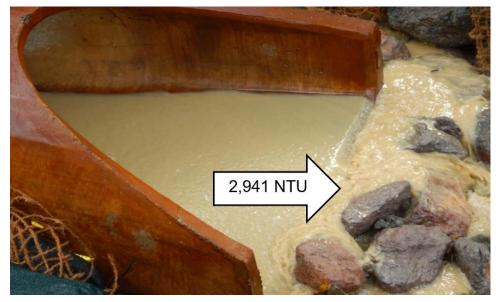
Figure 49. Highly turbid water (2,941 NTU) in stream due to failure by the Discharger to implement BMPs along Road 5. November 29, 2018.
