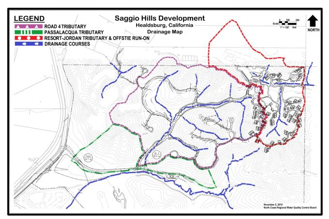
Figure 1. Saggio Hills construction site.
